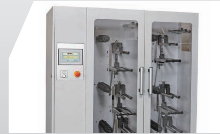
6 shafts rewinding Device
